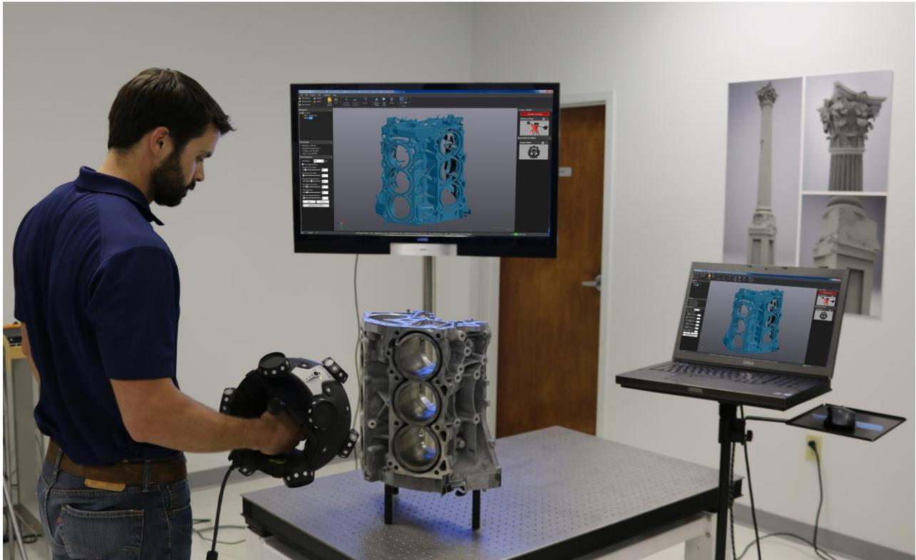
**Creaform MetraSCAN optically tracked 3D scanning and probing system**
